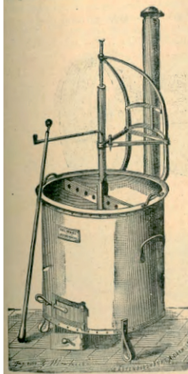
Fig. 12.5. Cauldron for cooking plum jam with its own firebox and stirrer
