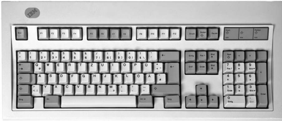
Fig. 34. IBM's Model M keyboard. German keyboard layout (QWERTZ, ISO-DE)
