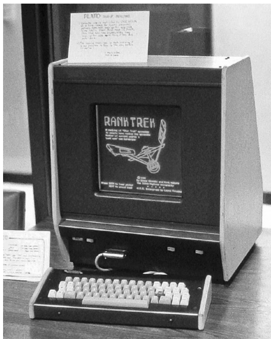
Fig. 12. PLATO V Terminal with plasma display, 1981
